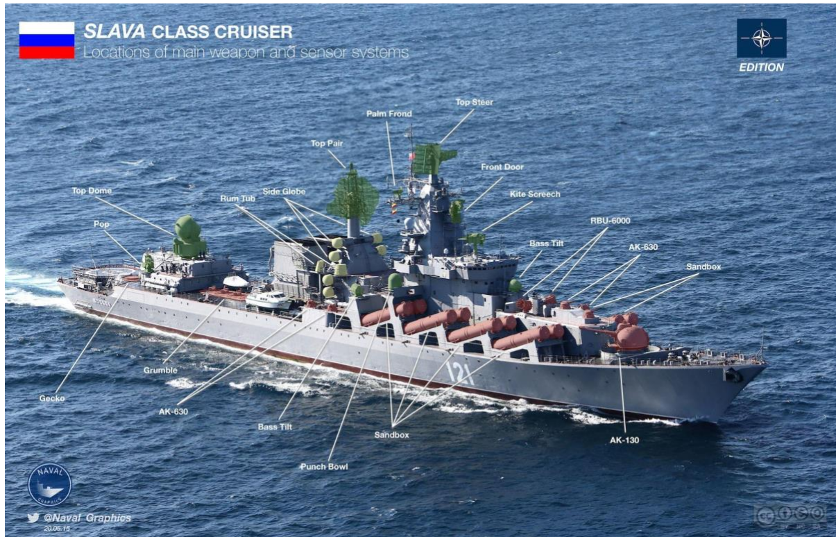
Figure-2: Moskva's sensors and weapons, Source: Naval Graphics
